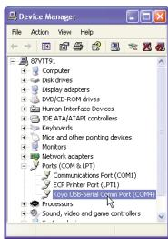
COM4 is the USB port used in this example. If you cannot find the Koyo USB-Serial Comm Port under Ports (COM & LBT) in **Device Manager**, the USB driver may not be correctly installed or the driver has a problem. Disconnect the cable from the PC and follow these steps to re-install the driver:
