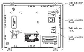
On either serial communications port, if there is no activity on one or both TxD and RxD LED status indicators, then it should be suspected that either:
