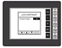
Press the F1 and F5 keys simultaneously for 3 seconds and the panel will bring up the the System Setup Screen menu. Select the Setting menu, and then select item 1; LCD Contrast. The default value is 8. Adjust the current value from 1 to 16 and the panel's contrast should become greater as the value moves toward 16 and it should become less as the value moves toward 1. If this does not happen, then the panel may need to be replaced. See note above.
