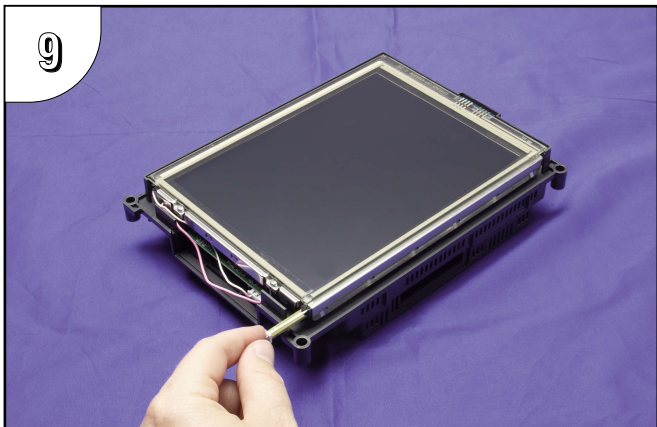
9 Position the replacement bulb so that the opening in its three-sided gold colored reflector faces toward the LCD touch screen. Using gentle pressure, slide the bulb into the guide until the retaining clip locks.
