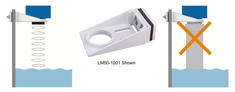
**Note:** The Side Mount Bracket (LM50 series) is not designed for use with stand pipes or as a method to secure stand pipes. There are too few threads to properly hold the sensor and the stand pipe.
