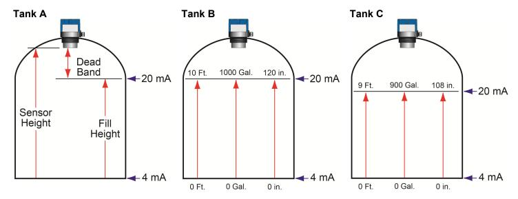
In the **Tank A** example, the Sensor Height sets the 4mA to the bottom of the tank. Fill-Height sets the 20mA to the top of the straight side of the tank.
