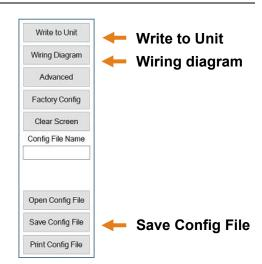
"Save Config File" will save this configuration as a text file which can be loaded back into WebCal® by pressing the "Open Config File" button. It is good practice to save the configuration file for each different configuration with a unique name for easy identification. If using multiple sensors in identical applications, then use of a single configuration file is recommended.
