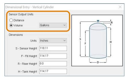
**Height:** Distance from the bottom of the tank to the top of the straight side wall.
