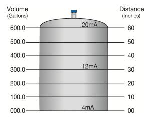
**Note:** In the above illustration, 10" of liquid will always be equal to 100 gallons of liquid (1" = 10 gallons).
