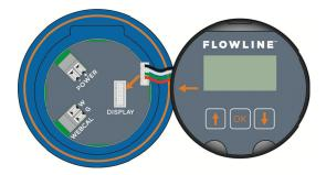
The sensor communicates to WebCal<sup>®</sup> through the USB<sup>®</sup> Fob. Prior to plugging the Fob into your computers USB<sup>®</sup> port, ensure that all external power is disconnected from EchoPod<sup>®</sup>. The maximum distance between the computer and EchoPod<sup>®</sup> is 15'.
