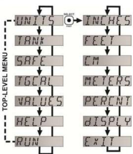
**Note:** EchoSpan<sup>®</sup> will adjust the display when measurement units are changed under **UNITS**. Example: If you are in inches and the display reads 60.0, the display will change to 5.00 when feet is selected as the unit of measurement.
