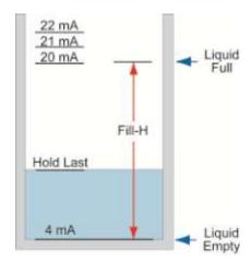
TG CAL – Target Calibration (allows for the sensor to accept as either EMPTY or FULL the liquid level at that moment. Liquid level must be at either the required EMPTY or FULL levels of liquid.
