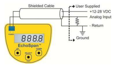
The cabling should be a shielded twisted pair to minimize EMI interference. Typically 20 to 24 gauge wire is used in this application.
