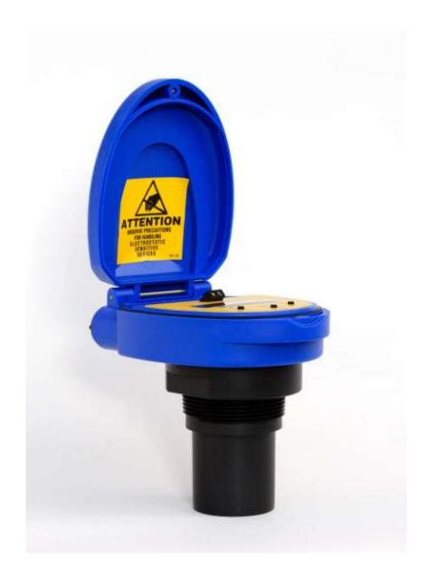
The EchoSpan<sup>®</sup> is a general-purpose ultrasonic level transmitter that provides a loop powered 4-20 mA output. The 4-20 mA output can be used to provide the proportional level of liquid in any tank or vessel. The signal can be connected to any device that accepts a loop powered 4-20 mA signal, such as a PLC, SCADA, DCS, display, controller, etc.
