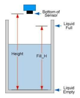
Before starting, take two measurements. 1) Measure the distance from the bottom of the sensor (transducer face) to the bottom of the tank. This will be the HEIGHT setting. 2) Measure the distance from the bottom of the tank to the Maximum Level of Liquid (Full). This will be the FILL-H setting.
