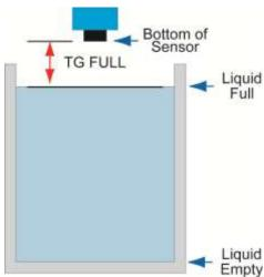
**TG Cal** is an alternative configuration method for setting the 4-20 mA current span within EchoSpan<sup>®</sup>. Use this method only if you are able to completely empty and/or fill the tank. TGCal involves two settings, Empty and Full.
