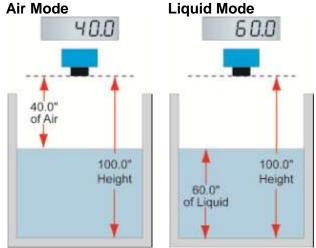
**Note:** Flowline recommends that when selecting **PERCNT**, configure the **HEIGHT** and **FILL-H** settings before selecting **PERCNT** in order to span the EchoSpan® for your application requirements. If **UNITS** is set to **PERCENT**, then **TANK** will not appear. To view **TANK**, set **UNITS** to any of the following: **INCHES**, **CM** (Centimeters), **FEET** or **METERS**.
