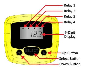
**Note:** To increase the scrolling speed of the display, hold down the SELECT button while simultaneously pressing the UP or DOWN button.
