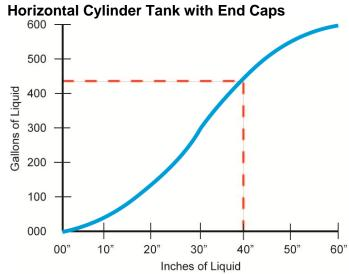
1" of liquid does not equal 10 gallons. The 10" at the bottom represents a rise of 62.8 gallons where the change between 10" and 20" represents an increase of 109.6 gallons.
