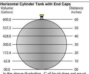
In the above illustration, 1" of liquid does not equal 10 gallons. The 10" at the bottom represents a rise of 62.8 gallons where the change between 10" and 20" represents an increase of 109.6 gallons.
