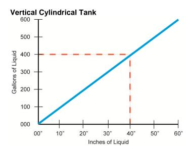
10" of liquid will always be equal to 100 gallons of liquid (1" = 10 gallons).
