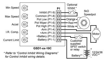
\*\* Select battery voltage as required per application and model specifications.
