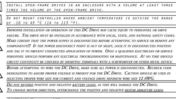
CAUTION!! TURN POWER OFF WHILE MAKING WIRING CONNECTIONS.
