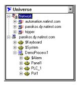
Each computer registered as running Lookout *Direct* appears in this dialog box. Clicking on the computer to open the full display reveals the processes currently running on that computer. Clicking on a particular process reveals all the objects in that process that you can access.
