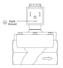
18 mm DIN Connector Power leads connected to vertical pins on all versions. Not polarity sensitive.
