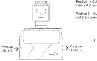
Position 1) Coil De-energized. Pressure inlet port (1) is closed to outlet port (2).
