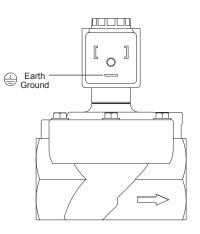
18 mm DIN Connector Power leads connected to vertical pins on all versions. Not polarity sensitive.
