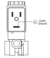
18 mm DIN Power leads connected to vertical pins on all versions. Not polarity sensitive.
