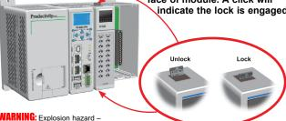
Do not connect or disconnect connectors or operate switches while circuit is live unless the area is known to be non-hazardous. Do not hotswap modules unless the area is known to be non-hazardous.
