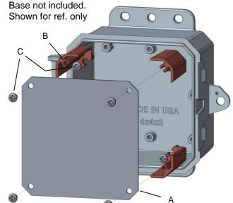
Position the Faceplate supports (B) (x4) flush against the inside wall of the Base and secure with #8-18 X 3/8" Pan Head Screws (C) (x4) into the hexagonal boss, as shown. Position the Faceplate panel (A) over the supports and secure with #8-18 X 3/8" Pan Head Screws (C) (x4) into the supports (B). Torque to 8-10 in-lbs., using Philips head #2 screwdriver.
