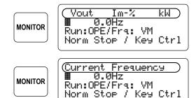
When the source of Frequency Setting is the Operator Keypad (OPE), the second line becomes dedicated to displaying the set frequency and actual frequency (preconfigured variable 2 output is suppressed). This feature is useful to help machine operators avoid severe frequency over-shoot / undershoot when the set acceleration and deceleration rates are relatively low.
