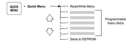
**Read/Write Menu** The Read/Write menu is located at the top of the Quick Menu list. It is necessary to use the Read/Write menu when you want to copy one inverter's parameters to another inverter. See "Copying Parameters Between Inverters" on page 3–26.
