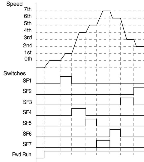
The following table lists the option codes for assigning [SF1 to [SF7] to the intelligent inputs.
