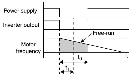
Inverter trips when  $t_0 > t_1$
