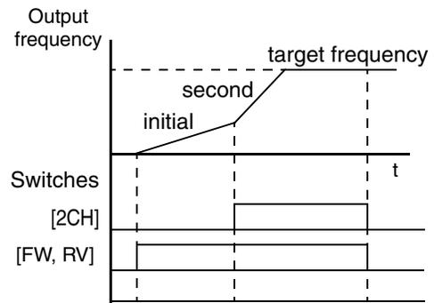
In the graph shown above, the [2CH] signal becomes active during acceleration. This causes the inverter to switch from using acceleration 1 (F002) to acceleration 2 (A092).
