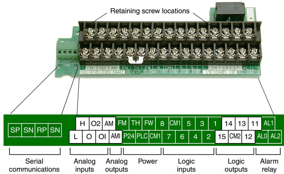
Specifications for the logic connection terminals are in the following table:
