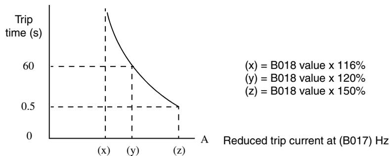
**Thermal Warning Output** – Using parameter C061, you can set the threshold from 0 to 100% of trip level for turning ON the intelligent output [THM] at that level. In this way, the inverter provides an early warning before the electronic thermal overload trips and turns OFF the output to the motor.
