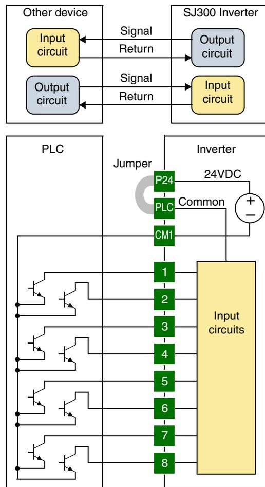
**Example Wiring Diagram**
