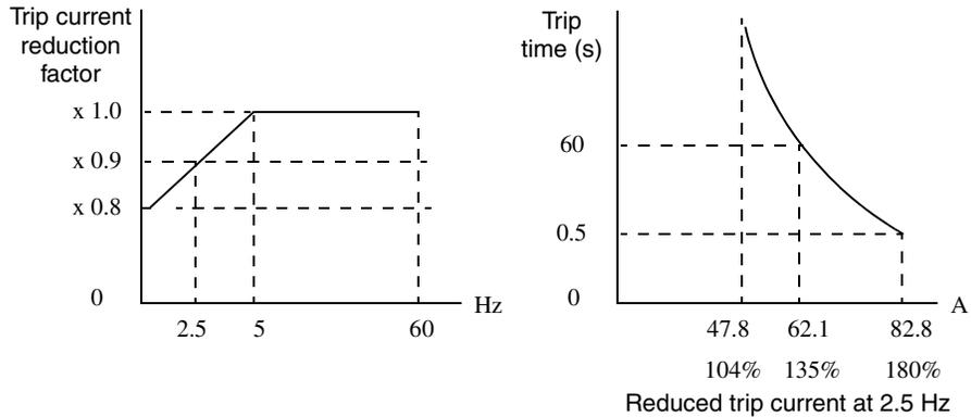
**Free Thermal Characteristic** - It is possible to set the electronic thermal characteristic using a free-form curve defined by three data points, according to the table below.
