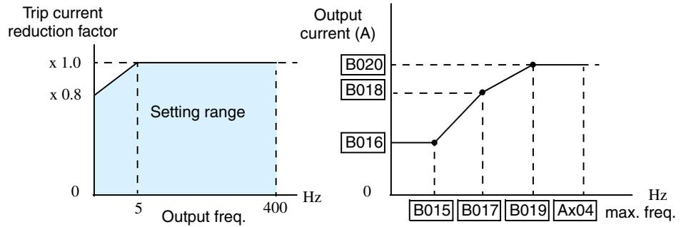
Suppose the electronic thermal setting (B012) is set to 44 Amperes. The graph below shows the effect of the free setting torque characteristic curve. For example, at (B017) Hz, the output current level to cause overheating in a fixed time period is reduced to (B018) A. Points (x), (y), and (z) show the adjusted trip current levels in those conditions for given trip times.
