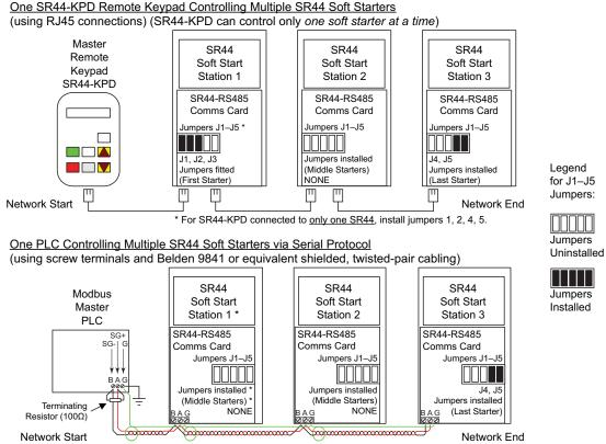
\* The 'Network Start' terminating resistor is installed at the PLC, and Station 1 is jumpered as a 'Middle Starter'. \* For RS-485 connection to <u>only one SR44</u>, install jumpers 4, 5.
