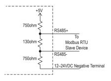
The external Modbus RTU device should share the same power supply reference (12–24 VDC negative terminal) as this device, or it must have an isolated RS-485 communications port.
