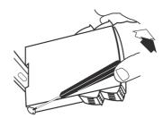
Max. wire size 1 x 2.5 mm2 stranded wire. Screw terminal torque 0.5 Nm.
