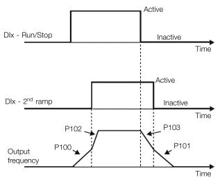
Figure 9.14: Example of the 2<sup>nd</sup> Ramp function
