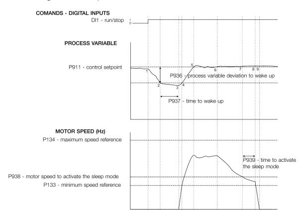
Figure 14.4: Operation of the PID controller with the sleep mode enabled
