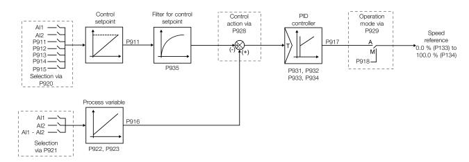
Figure 14.1: PID controller block diagram
