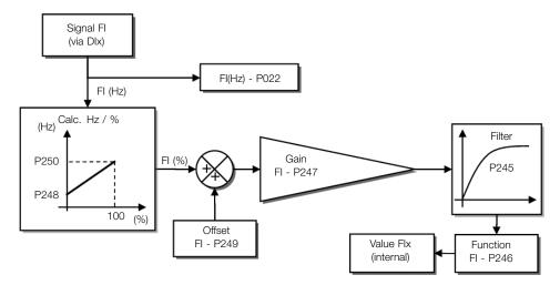
Figure 9.5: Block diagram of frequency input - FI (DIx)
