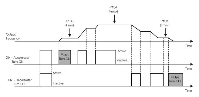
Figure 9.15: Example of the Accelerate Turn ON / Decelerate Turn OFF
