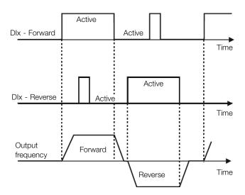
Figure 9.9: Example of the Forward /Reverse command
