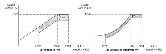
Figure 8.19: (a) and (b) Example of voltage behavior in V/f and quadratic V/f
