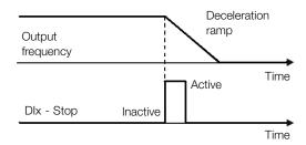
Figure 9.16: Example the stop function
