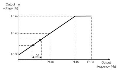
Figure 8.18: Slip compensation in an operation point of the standar V/f curve
