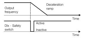
Figure 9.17: Example of the Emergency function
