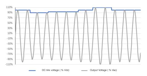
Figure 8.2: Influence of the DC Link in the output voltage
