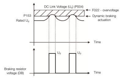
Figure 8.10: Dynamic braking actuation curve
