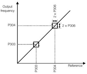
Figure 8.11: Actuation of the skip frequency
