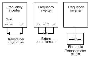
Figure 15.1: Connections for analog inputs
