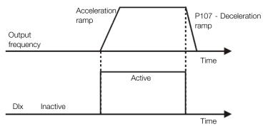
Figure 9.8: Example of the Quick Stop function
