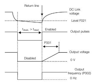
Figure 8.7: Actuation of the Ride-Through function
