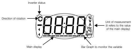
Figure 5.1: Screen on initialization and display fields
