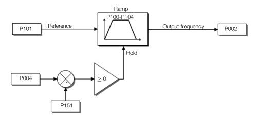
Figure 8.3: Block diagram DC Link voltage limitation
