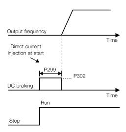
Figure 8.8: DC Braking actuation at start
