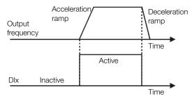
Figure 9.6: Example of the Run/Stop function
