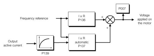
Figure 8.17: Block diagram of the automatic torque boost
