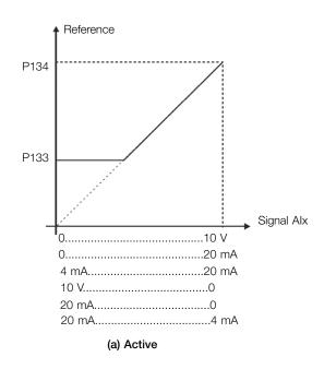
Figure 9.2: (a) and (b) Actuation of the analog inputs with dead zone
