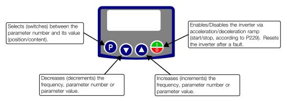
Figure 4.1: HMI keys
