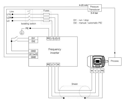
Figure 14.2: Example of the PID controller application
