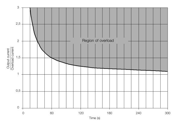
Figure 10.2: Actuation of the motor overload
