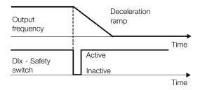
Figure 9.17: Example of the Emergency function
