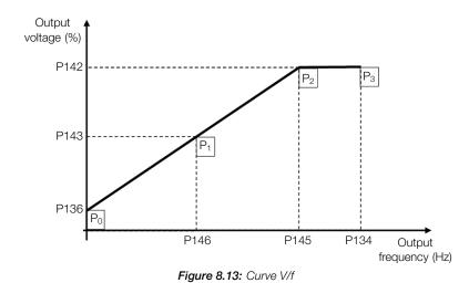
The factory default setting of the frequency inverter defines a linear relation of the torque with the frequency by means of three points  $(P_0, P_1 \text{ and } P_2)$ .
