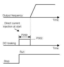
Figure 8.8: DC Braking actuation at start
