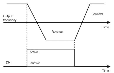
Figure 9.11: Example of the Direction of Rotation function
