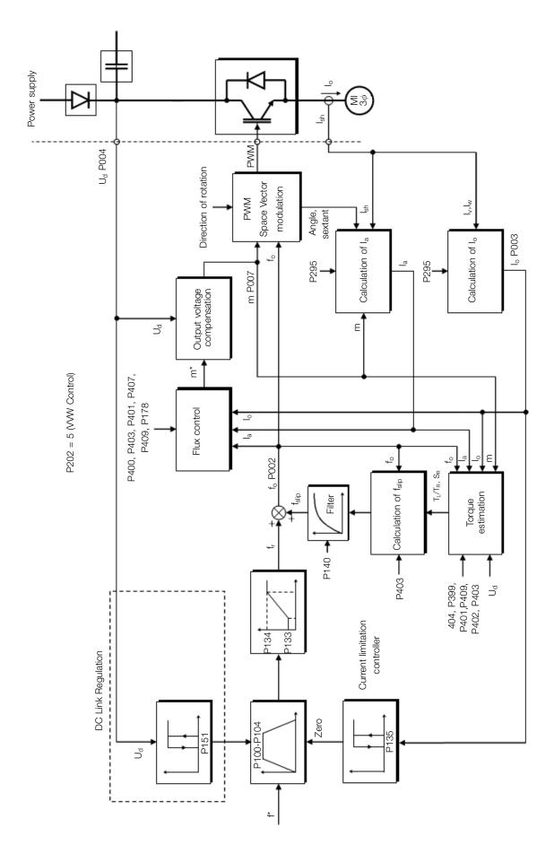
Figure 8.20: VVW control flow
