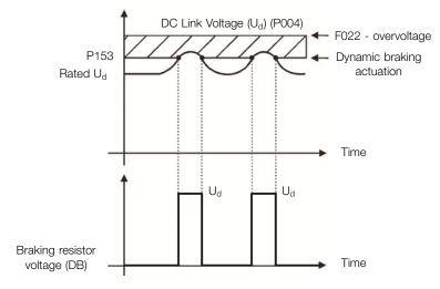
Figure 8.10: Dynamic braking actuation curve
