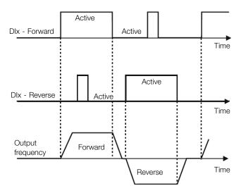
Figure 9.9: Example of the Forward /Reverse command
