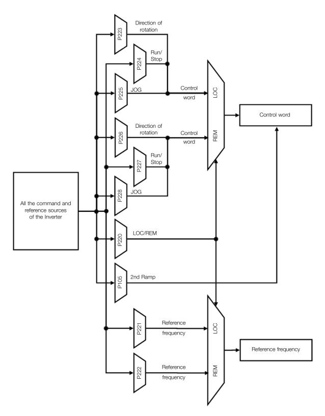
Figure 7.1: Block diagram for commands and references
