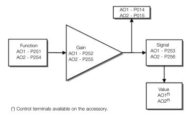
Figure 9.4: Block diagram of the analog output (AOx)
