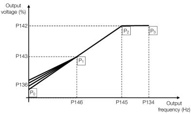
Figure 8.15: Torque boost region for quadratic V/f control mode
