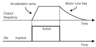
Figure 9.7: Example of the General Enable function
