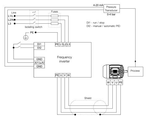
Figure 15.7: Example of the PID controller application
