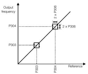
Figure 8.11: Actuation of the skip frequency
