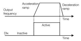
Figure 9.6: Example of the Run/Stop function
