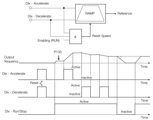
Figure 9.13: Example of the Electronic Potentiometer (E.P.) function
