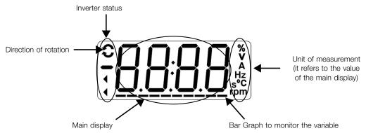
Figure 5.1: Screen on initialization and display fields
