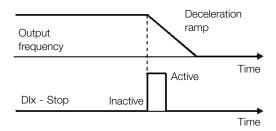
Figure 9.16: Example the stop function
