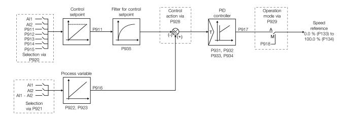
Figure 14.1: PID controller block diagram
