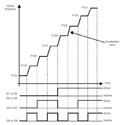
Figure 7.3: Operating graph of the Multispeed function
