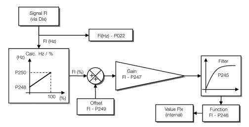
Figure 9.5: Block diagram of frequency input - FI (DIx)
