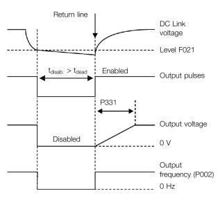
Figure 8.7: Actuation of the Ride-Through function
