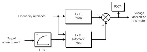
Figure 8.17: Block diagram of the automatic torque boost
