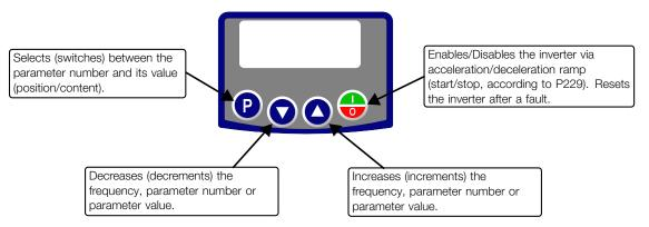
Figure 4.1: HMI keys
