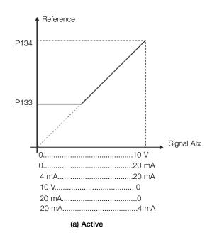
Figure 9.2: (a) and (b) Actuation of the analog inputs with dead zone
