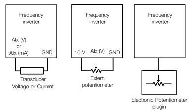
Figure 15.1: Connections for analog inputs
