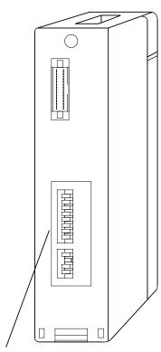
DIP Switches for communications and Protocol Setup
